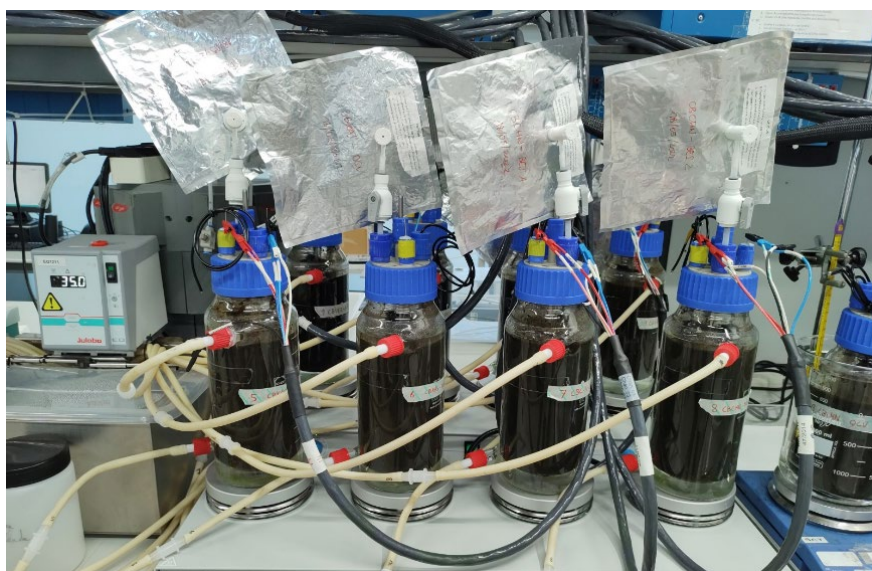
Figure 8 - Laboratory set-up for activity 2 with 6 1L reactors available at mesophilic conditions and connected to gas collector bags
